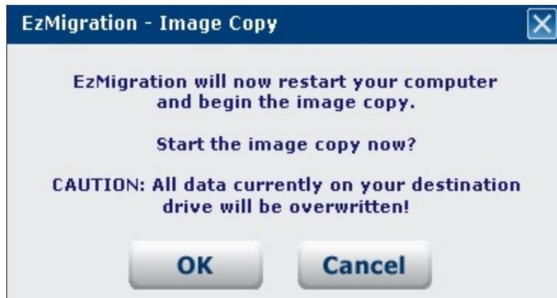
EzMigration will restart your computer and begin to create an image copy (an exact duplicate) of your SOURCE drive on the new drive. The image copy will overwrite the **entire** DESTINATION disk. This means that any existing data on the DESTINATION drive will be destroyed.
